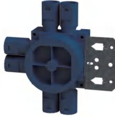
Single wall box for double plasterboard with Ø16/Ø20mm inlets and adjustable fixing plate
